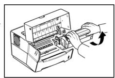
2 Using the green handles lift the Drum Unit out of the machine.
